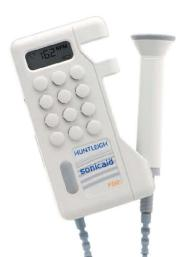
This top of the range handheld rate display Doppler features high sensitivity interchangeable probes. 2MHz for general obstetric use, 3MHz ideally suited for detecting the fetal heart in early gestations.
